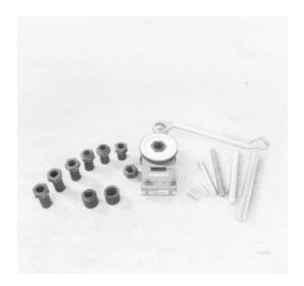
Anchor test gauge with thread adapters and threaded rods, a ring wrench, spacer and intermediate spacer.
