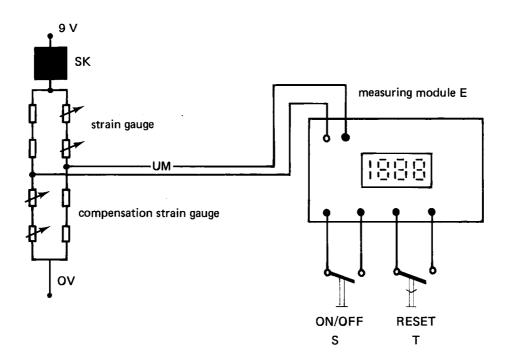
The four strain gauges that are bonded to the measuring ring combined with the four compensation strain gauges that are adhered to a square section, form a Wheatstone bridge. The diagonal voltage, that is described as the measuring voltage, UM, is amplified by the measuring module, E, and shown in kN by the LCD indicator, A.
