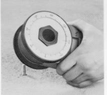
The gauge can be The gauge can be The thread adapter connected straight to is screwed on and the HSA (HKB), HVA connects the anchor (adhesive) and HSLG to the gauge. heavy-duty stud anchor. The central bore is placed over the protruding threaded section of the anchor.
